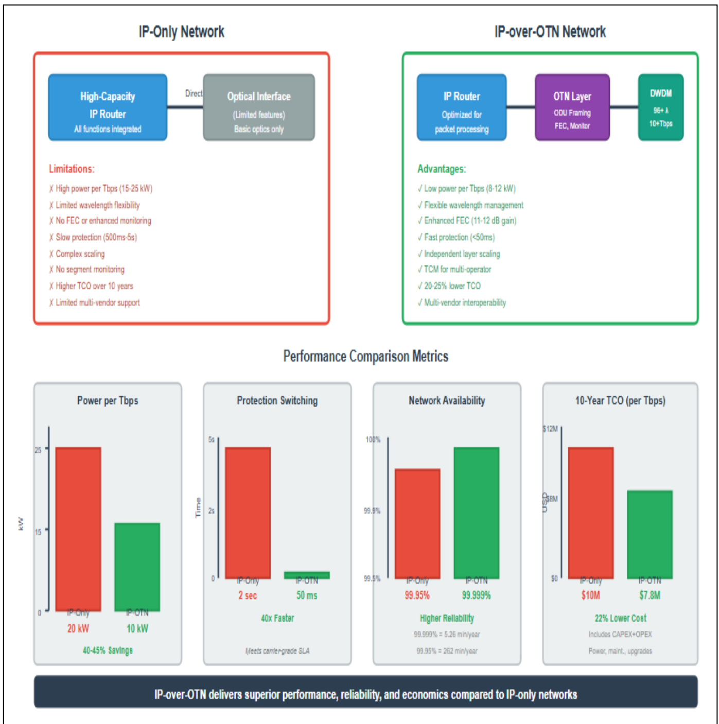
Fig 6 Comparative Analysis - IP-Only vs IP-over-OTN Networks
