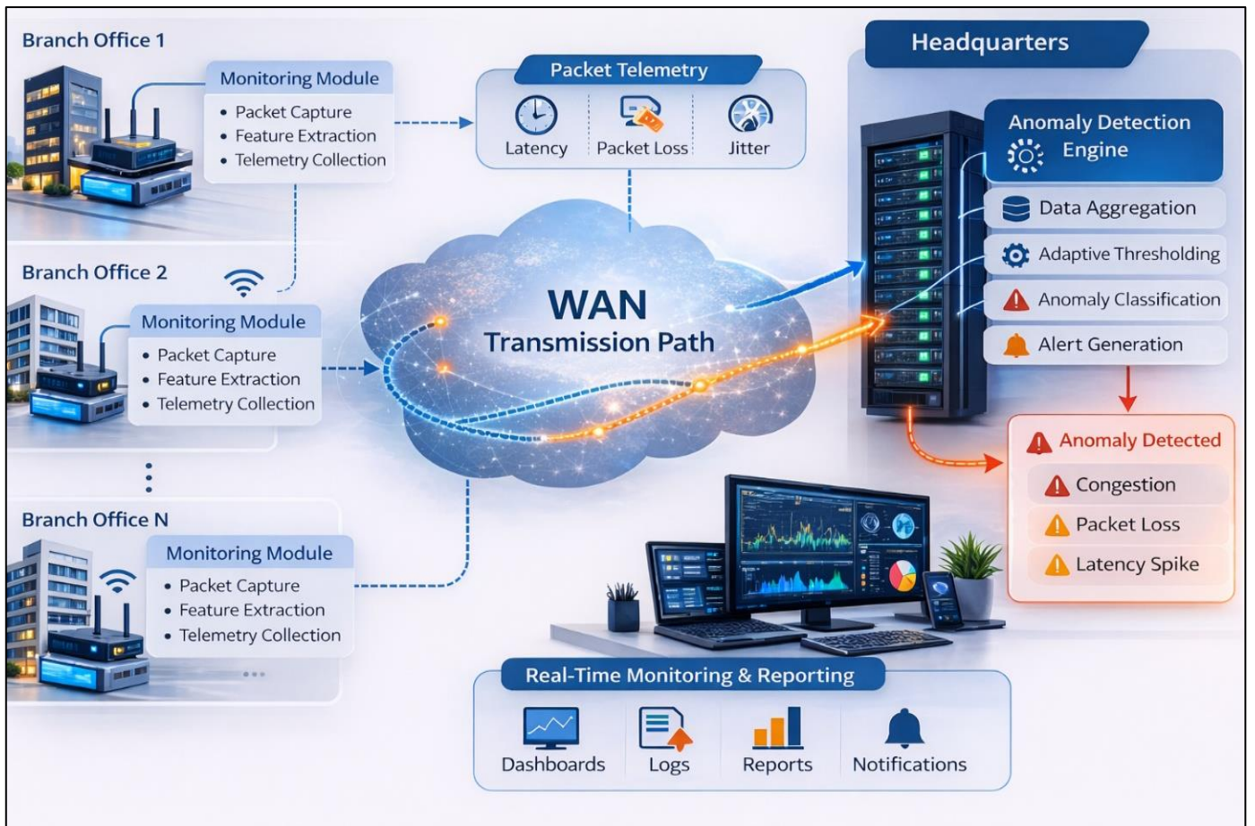
Fig 1 Architecture of the Adaptive WAN Link Anomaly Detection Framework for Branch-to-HQ Networks
