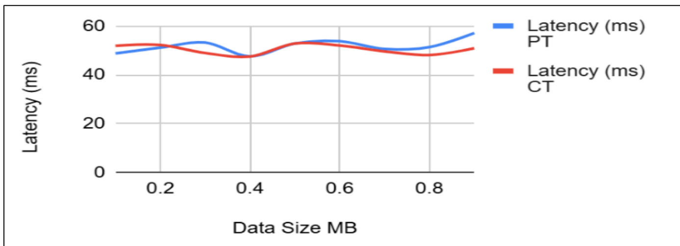
Fig 4b Latency for Plain and Cipher Text for Data Size (0.1 – 0.9) MB.
