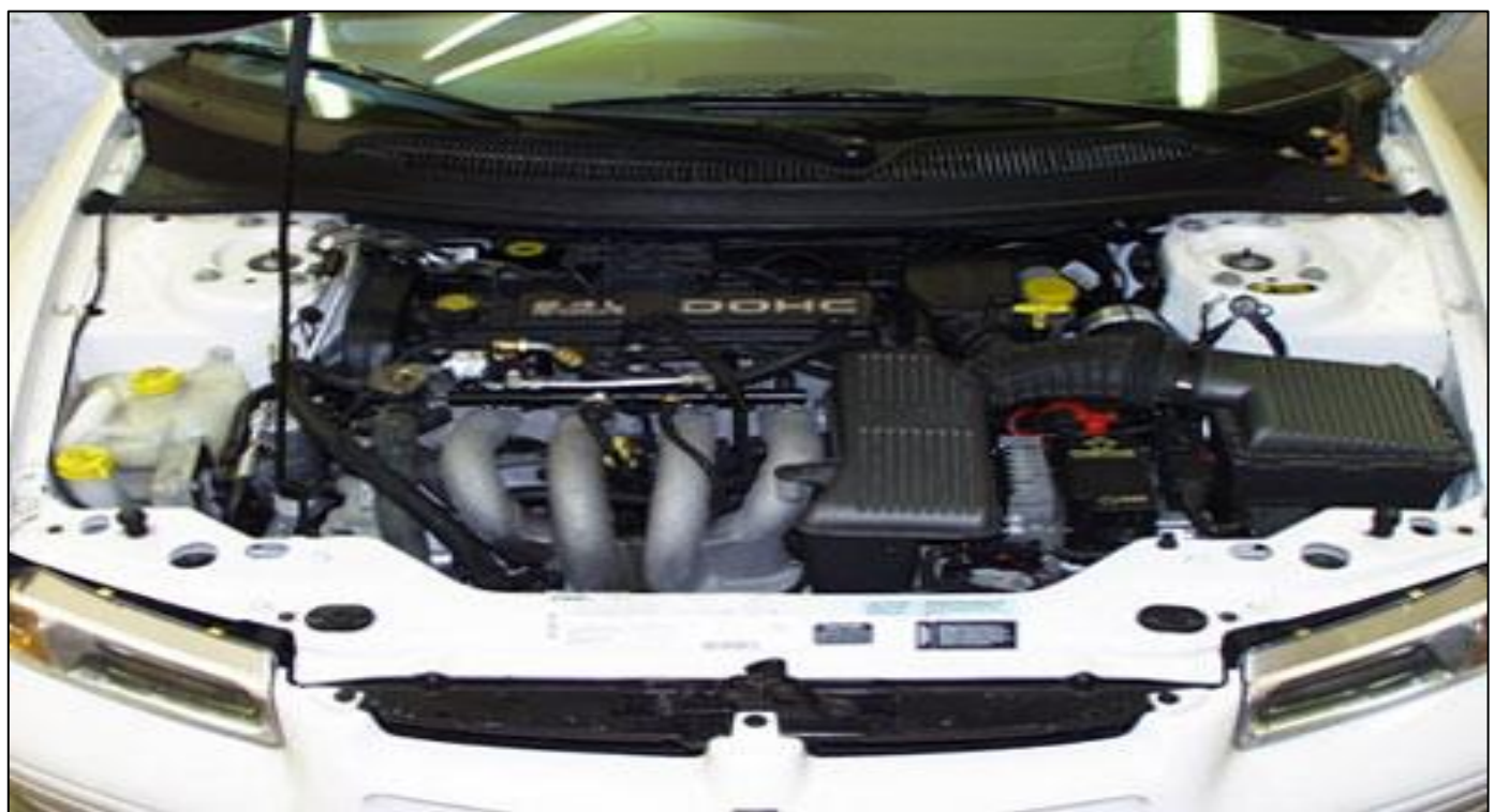
Fig 4 an installed CNG engine (Dedicated)
